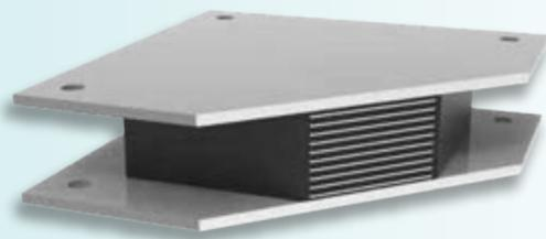
Arfen elastomeric (rubber) bearings consisting of waterproof rubber and steel shim are used to transfer the load from superstructure to the bridge pier accurately and directly. This system is made of natural rubber (NR) or chloroprene (CR) and steel plate (shim) (in F type only rubber is used.)
