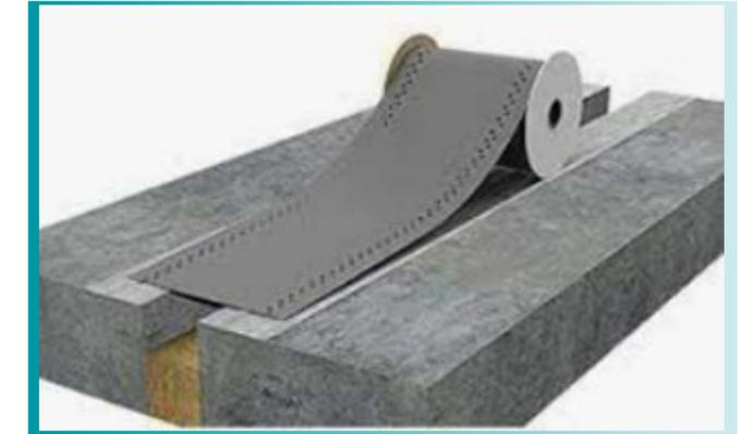
HYDROFLEX is a highly elastic dilatation tape used in the insulation of dilatation gaps, thermal expansion joints and cracks. It is produced in 150 mm - 200 mm - 250 mm - 300 mm - 400 mm widths with or without holes, in 1 mm, 1,50 and 2 mm thicknesses.
