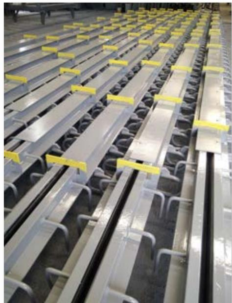
Arfen single-span steel expansion joints are used in transverse direction at the bridges, with a total movement capacity of 80 mm or 100 mm, the bearing assembly is connected to the structure by means of the ropes and the rubber strip sealing element for water tightness is used. The steel profiles in this system can consist of extrusion profiles.
