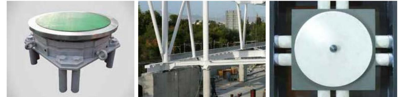
This type isolator works with the energy damping principle by friction. If the seismic forces acting on such isolators exceed the static frictional force limit, the steel sphere in the isolator begins to slip on the concave bottom plate. Then the isolator allows the structure to oscillate like a pendulum.
