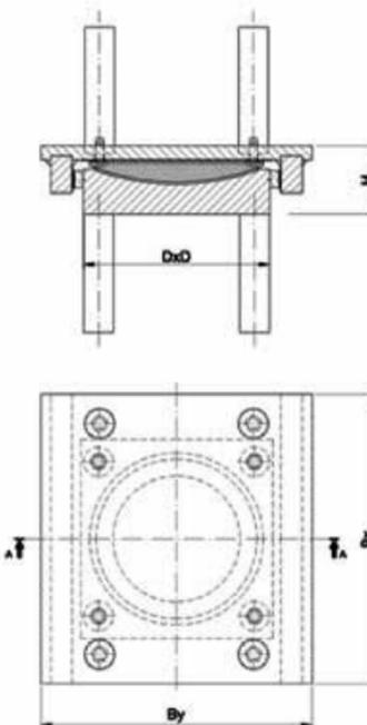
The technical data is shown in the table for guided spherical bearings. For example, AGSFL500/100-75 means the vertical load is 500 kN, the longitudinally transversal displacement is 100 mm (±50), and transversal (or longitudinal) lateral load is 75 kN.
