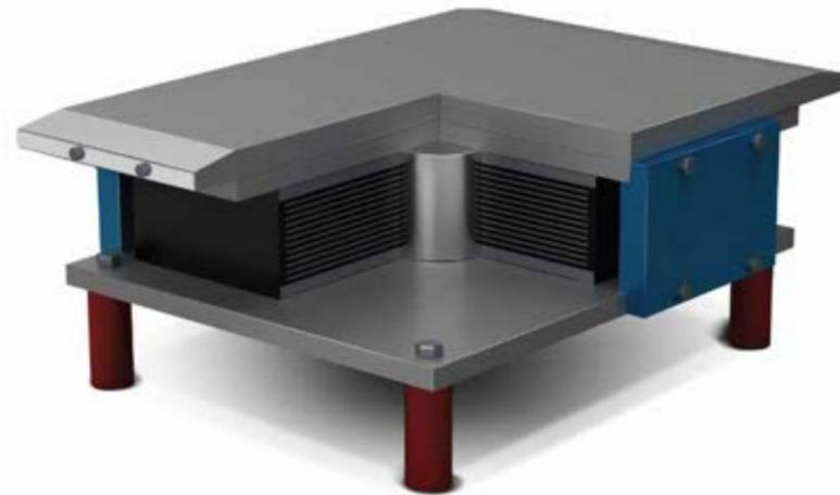
The damping capacity is increased by adding extra materials to the natural rubber. High damping rubber bearings consist of reinforced multilayers with steel plates between HDRB specially compounded damping rubber and rubber layers. Steel plates provide vertical rigidity and rubber horizontal flexibility. They can be made rectangular or circular accordance to client request.
